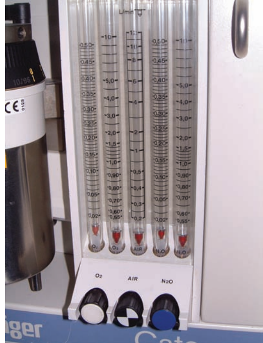
Figure 2.11 Oxygen, air and nitrous oxide flowmeters on an anaesthetic machine.
